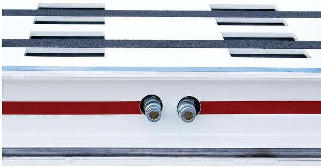
Quick connect no-drip hydraulic couplers, four each side, eight total.
