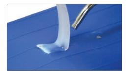
The NP-3 Plastic Welder is designed to use nitrogen gas as a heating source. By using nitrogen instead of compressed air we accomplish a much cleaner bond of the plastic with no contamination such as oxygen. The weld strength is much stronger than using air or any adhesive. By melting the plastics and fusing the repair with the same material as the base material, there is no contamination or oxidation problems, thus achieving very strong repairs.
