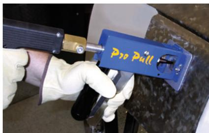
Pro Pull Dent Pulling. Position the weld tip in the bottom of the dent, weld, then squeeze the handle to initialize the pulling action.
