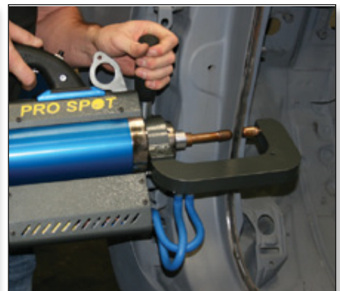
Spot welding of quarter panel using C-Arm
