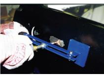
Lever bar welding. Simply weld on the shaft to the dent and pull the lever to straighten.
