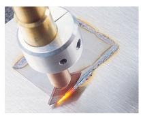
Ideal for rust repair and patching, stitch welding works by delivering an intermittent or pulsating current while rolling the tip in the sheet metal edge.
