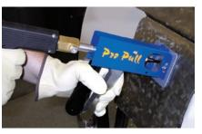
Pro Pull Dent Pulling. Position the weld tip in the bottom of the dent, weld, then squeeze the handle to initialize the pulling action.
