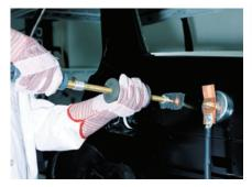
Quickest dent pulling system ever! Just weld on the hammer directly on the dent and hammer away. Simply twist to release. (magnetic ground plate optional)
