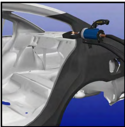
Spot welding of quarter panel using C-Arm (PS-302).
