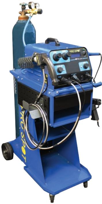
The unique feature with the NP-3 is that it is designed to save nitrogen gas costs. Because the unit requires a constant flow of air through the heating tube (or it will overheat and damage the heating element), the NP-3 blows compressed air thru the gun until you push the weld trigger then it automatically switches to nitrogen gas; when the weld trigger is released, it switches back to air. This saves a lot of waste of nitrogen gas, as it's only used when it's needed.
