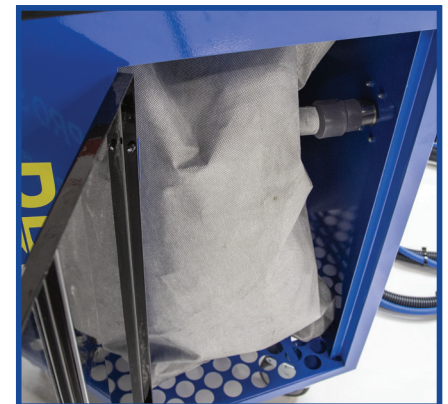
Accessible Side Doors for Fast Filter and Vacuum Bag Changes
