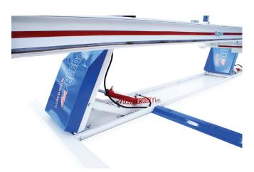
Working height, 14 in. up to 41 in.. Lowers to a loading height of 12 in.
