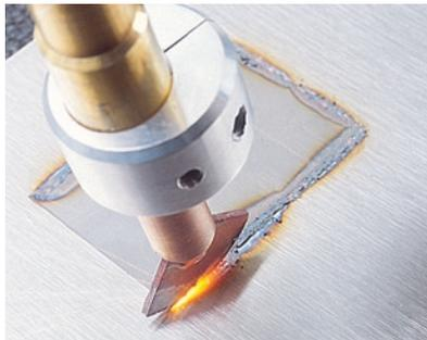
Ideal for rust repair and patching, stitch welding works by delivering an intermittent or pulsating current while rolling the tip in the sheet metal edge.
