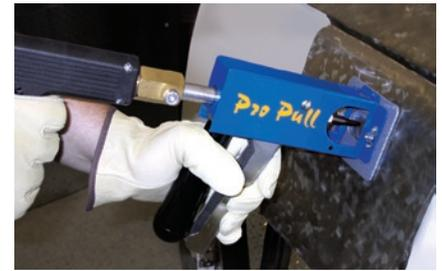
Pro Pull Dent Pulling. Position the weld tip in the bottom of the dent, weld, then squeeze the handle to initialize the pulling action.
