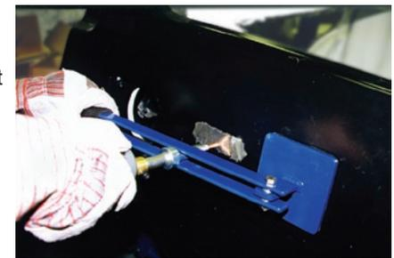
Lever bar welding. Simply weld on the shaft to the dent and pull the lever to straighten.
