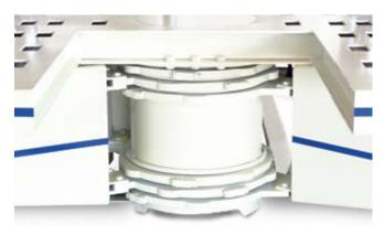
Three towers pivot from the large drum which also stores the electric over hydraulic pump.
